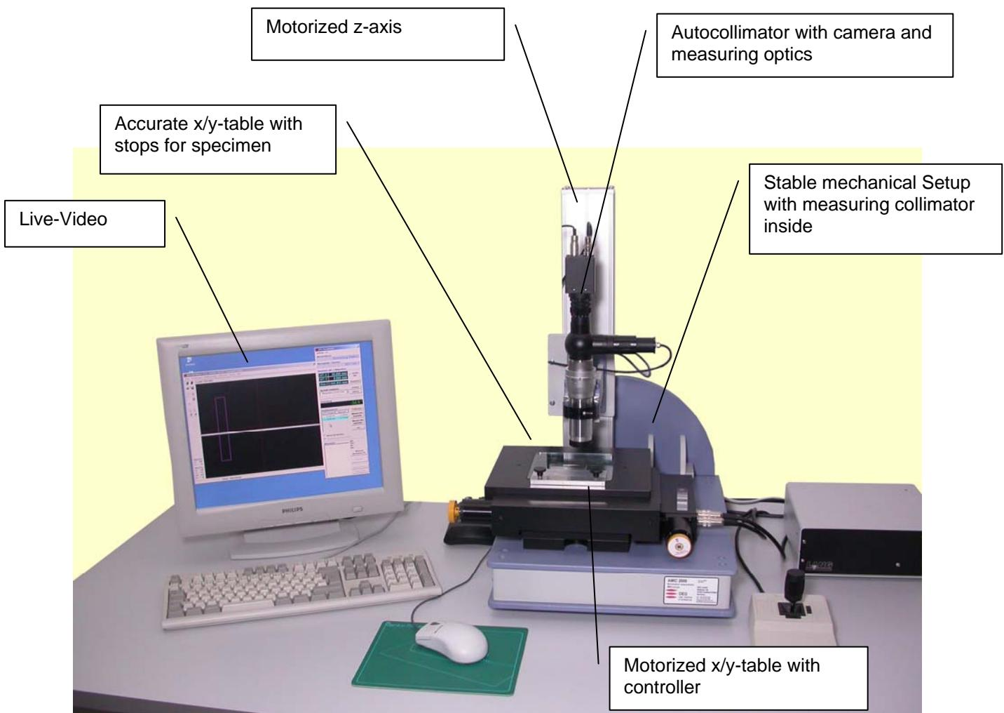
**OTS-Z** is a computer controlled measuring instrument for optical and geometrical parameters of cylindrical lenses. It is characterized by automatic measuring sequences for numerous parameters, a large measuring range and a simple operation. **OTS-Z** is suited for the most measuring tasks, which appear in practice. **OTS-Z** supplies accurate measuring results in short measuring times.
