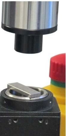
Using a gauge block, a reference to the flange of the camera housing is made. The reference value is stored. As second step the position of the chip can be directly measured in relation to the reference. The pixels of the chip can be seen clearly (see pic. below).
